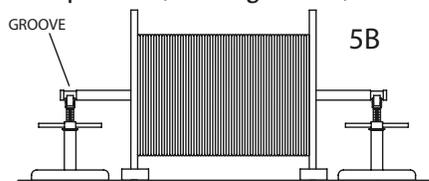
**NOTE:** Depending on the beginning spindle height, it may be necessary to elevate the telescoping square tubing of the reel stand. Manually lift the telescoping square tubing to the desired height and insert the pin(s) provided.
